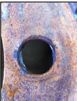
**Left: Rusted out wheel and lug hole on snow plow. Wheels and tires on the plow were recently replaced. Brake systems were also overhauled.**
