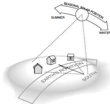
If the building in the middle were longer, stretching toward the two houses located on either side of it, more of its mass would be ideally situated to absorb and radiate heat in the winter
