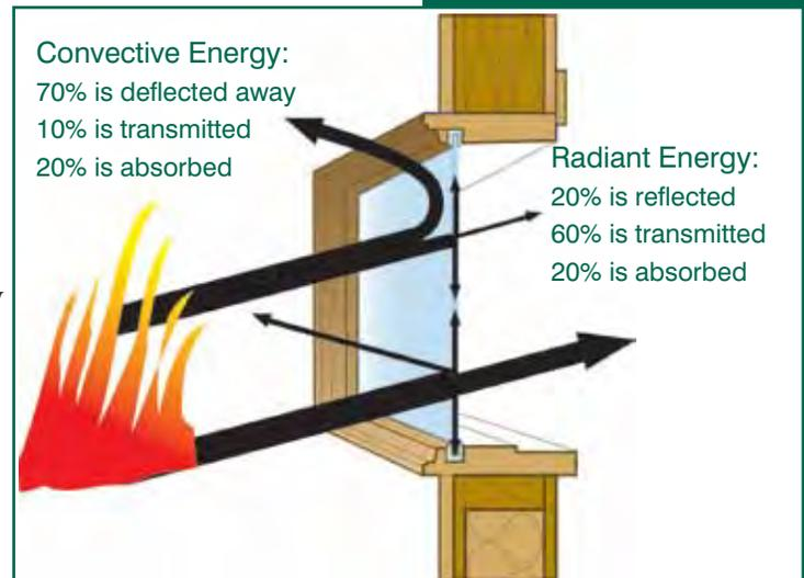
Figure 5-10: Energy transmission, conventional glass
