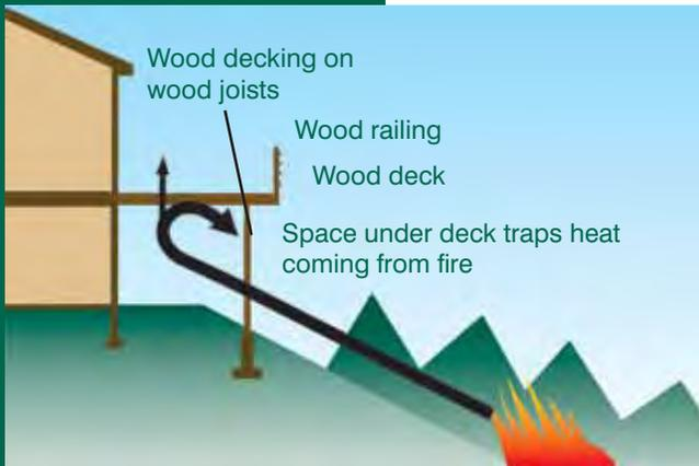
Figure 4-10: Conventional deck in a fire
