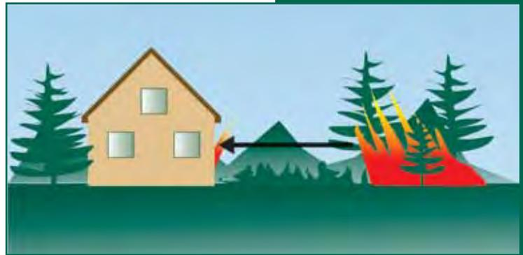
Figure 2-3: Radiant heating
