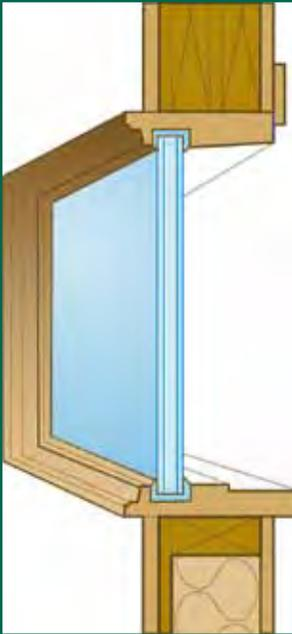
Figure 5-12: Thermopane window
