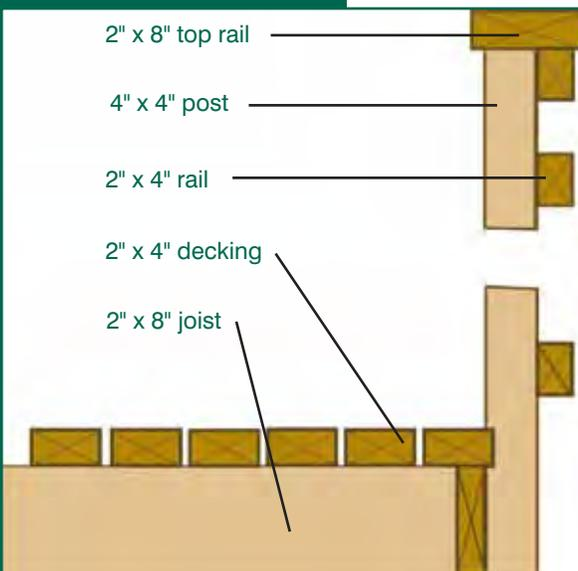
Figure 4-11: Conventional deck construction detail
