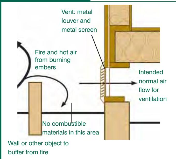
Figure 4-5: Crawl-space ventilation
